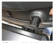
Place springs into locating holes on top of base.
